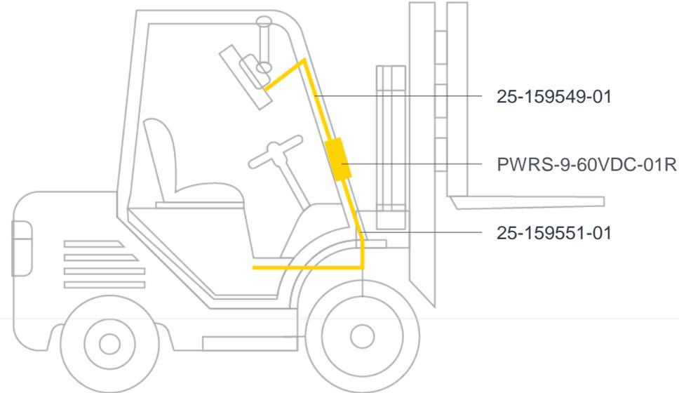
**VC70** **VEHICLE MOUNT (DC POWER SUPPLY NOT MOUNTED ON THE VC70)**
